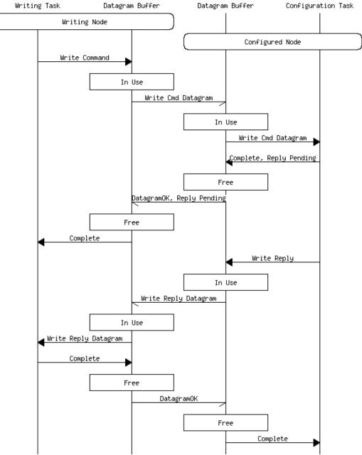
115 A delayed response, either because the write takes significant time or could fail for some reason. The datagram reply to the Write Command carries the reply pending bit set, and a reply datagram is send from the configured node back to the configuring node with the reply.
