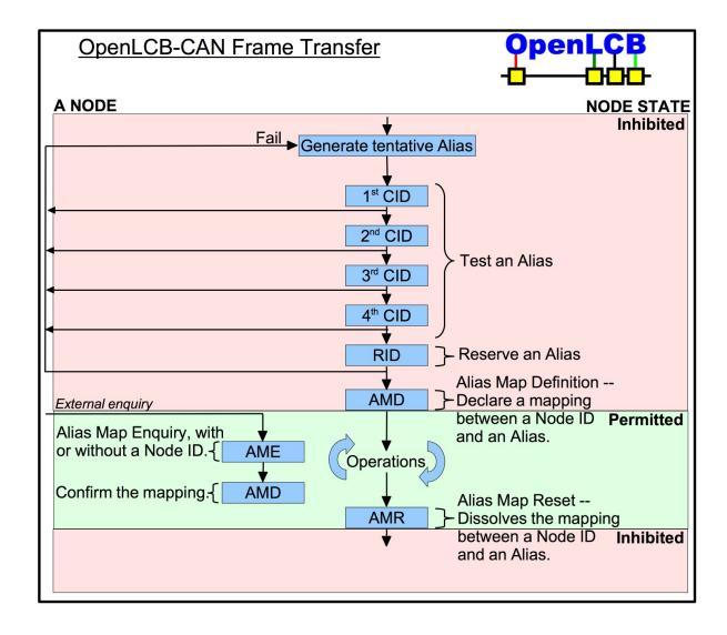
Note that in the diagram above, the 'Fails' are due to the node receiving a message which uses its tentative Alias, and it therefore needs to back off and try a new tentative Alias.
