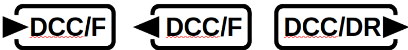
Figure 2: Example graphics depicting, from left to right, a DCC Full Scale Interface Consumer, DCC Full Scale Interface Source, DCC Driver/Receiver Interface Source. Other variations are also possible.
