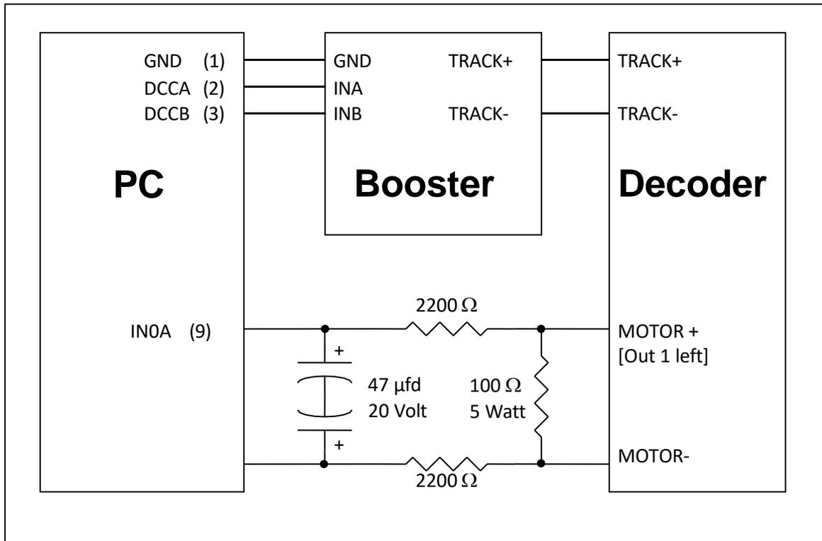
135 Locomotive decoders work by presetting the decoder to half speed reverse and then sending an emergency stop signal. The test must be able to tell the difference between half speed reverse and stopped. The test jig shown can reliably determine this change of state for all the locomotive decoders tested to date.
